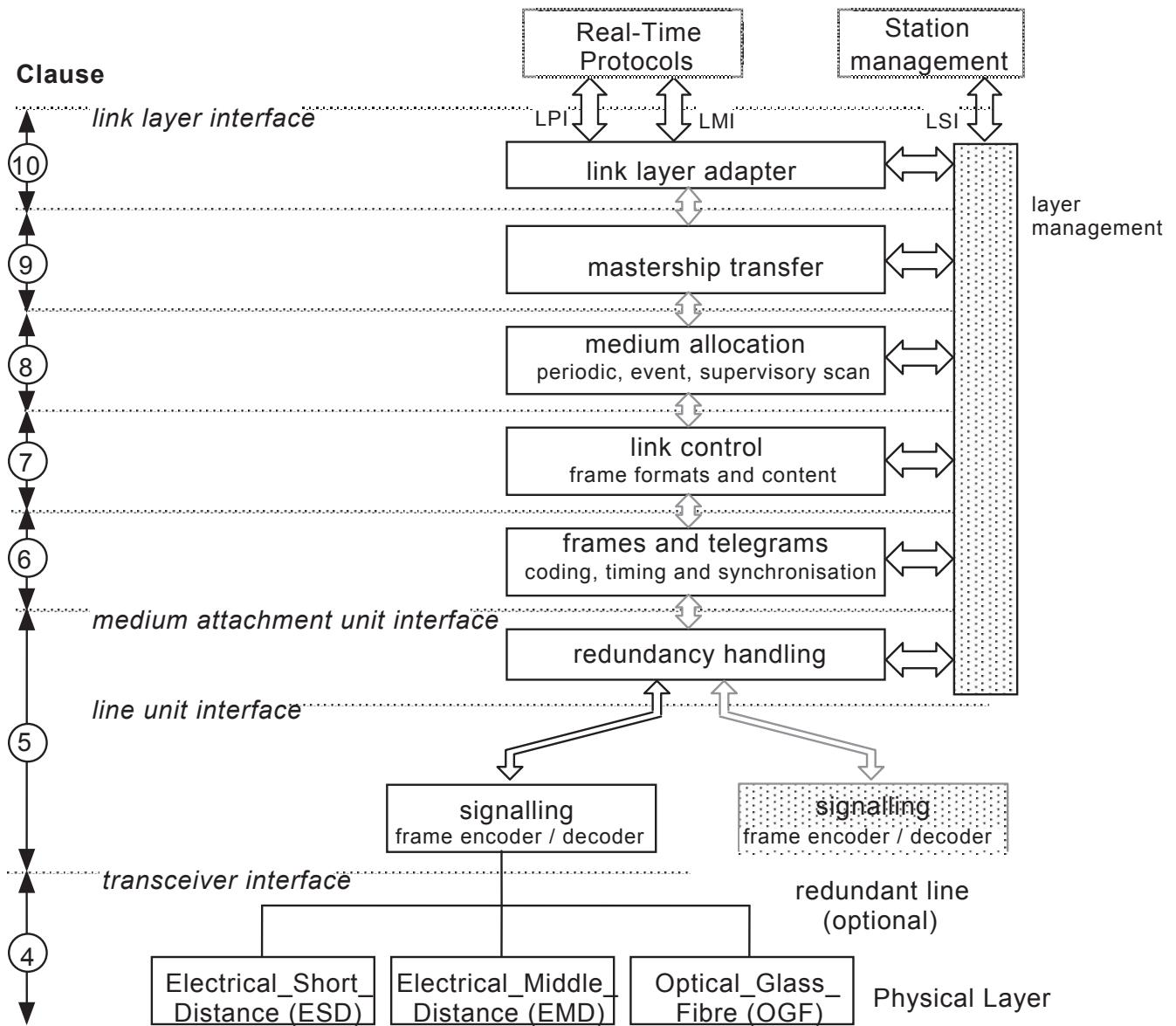
Figure 1 – Reference device and structure of the document
